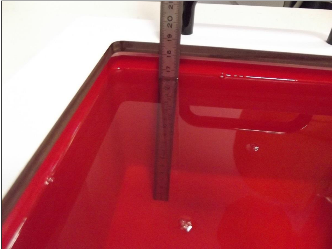
Photo 1: Liquid depth 450 MHz body simulating liquid
