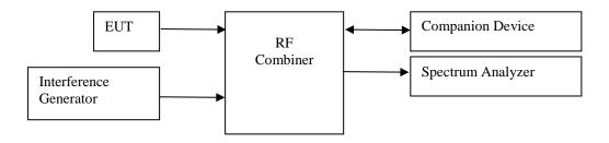
This test setup is used for all Monitoring and Time and Spectrum Access Procedure tests. The path loss from the signal generator to the EUT is measured with a power meter before the testing is started.
