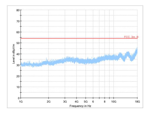
The radiated spurious emission of the unintentional radiator is below the indicated limit.
