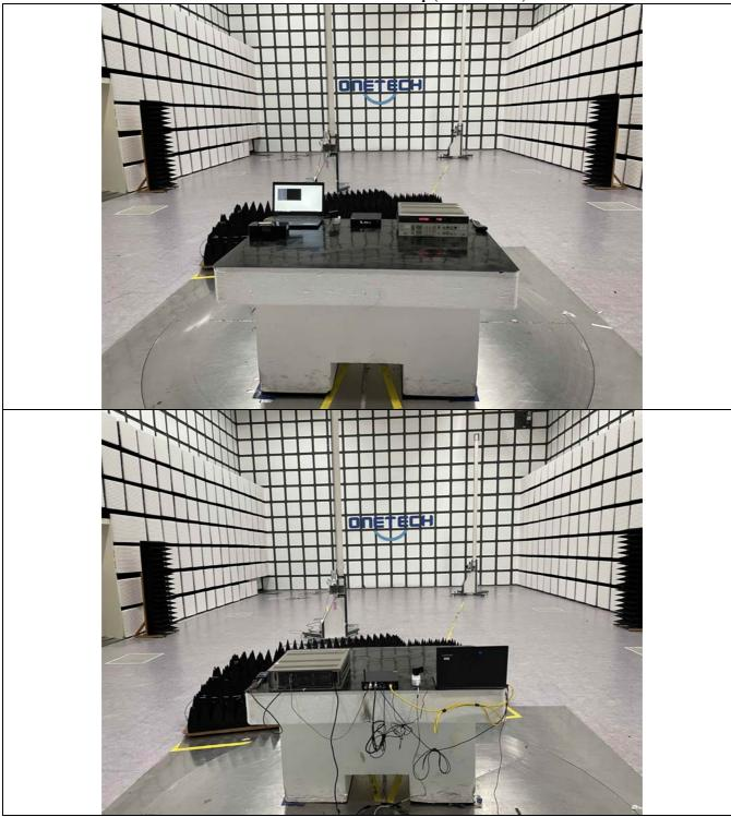
Radiated Disturbance Test Set Up (Above 1 GHz)
