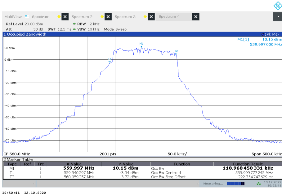
Plot 2: 560.000 MHz, max hold with frequency variation from 50 Hz to 15 kHz
