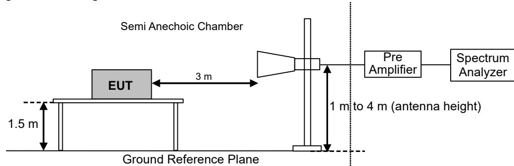
The carrier level and noise levels were confirmed at each position of X, Y and Z axes of EUT to see the position of maximum noise, and the test was made at the position that has the maximum noise.
