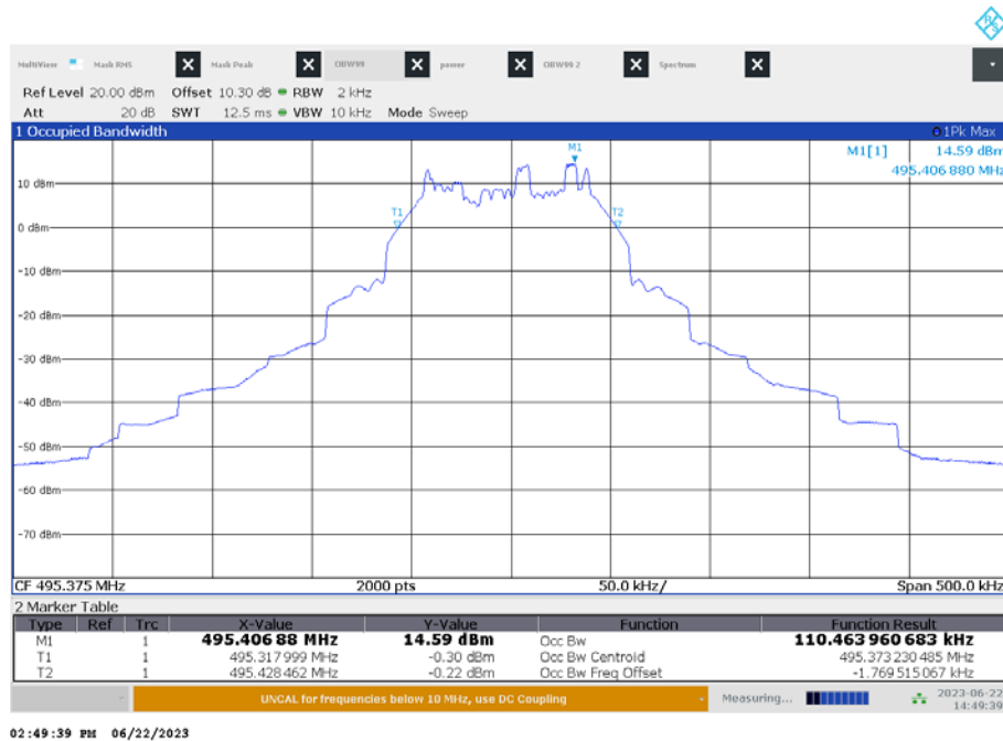
Plot 2: 495.375 MHz, max hold with frequency variation from 50 Hz to 15 kHz
