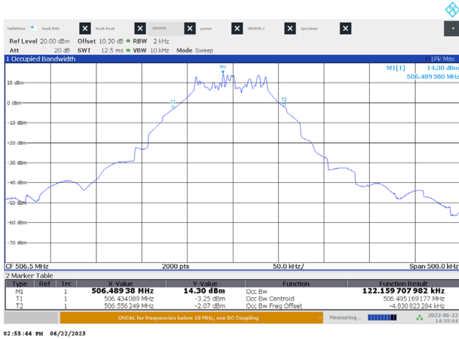
Plot 3: 506.500 MHz, max hold with frequency variation from 50 Hz to 15 kHz
