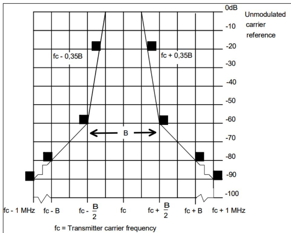
**Procedure:** KDB 971168 D01 Power Bandwidth 99% section 4.2
