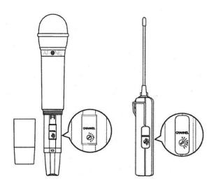
Adjust the transmitters to the same channel as the receiver. The label indicates the FIRST channel of the two frequency groups; '1' is equal to group 1 channel 11 with the other three channels followings. '2' is the beginning of the second frequency group.\*
