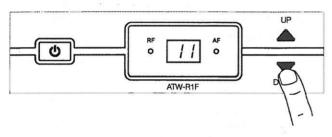
Press ▲ or ▼ and hold for 1 sec. The channel display begins flashing. Release and press ▲ (forward) or ▼ (backward) again to select an interference-free channel.
