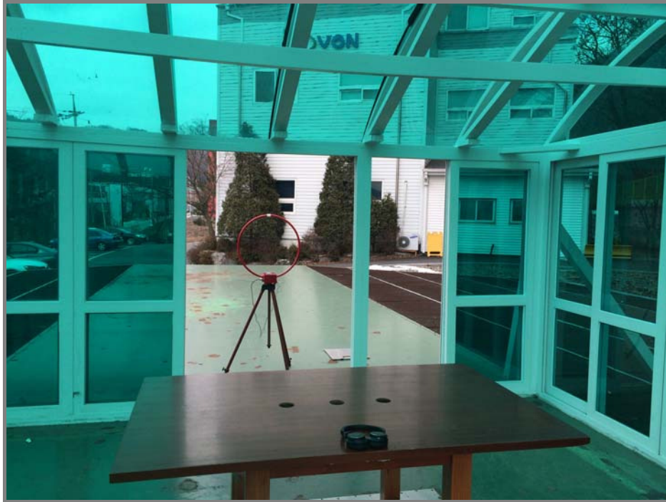
Photo of radiated spurious emission at below 30 MHz
