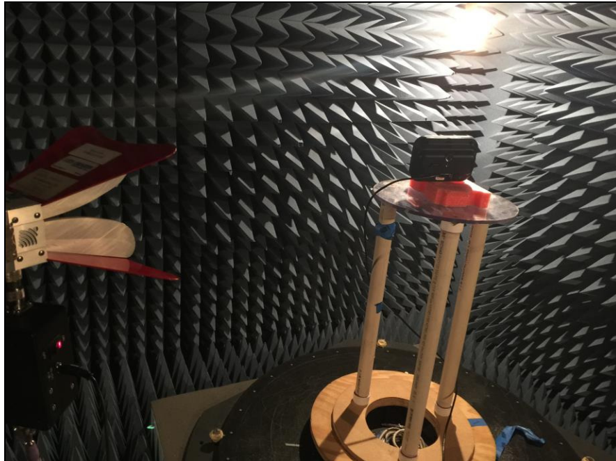
Photograph 2. Radiated Emissions, Test Setup, Above 1 GHz
