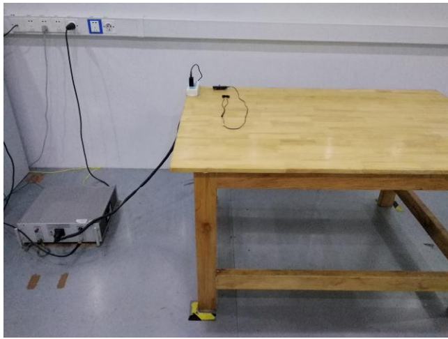
Conducted Emissions Test Setup Front View
