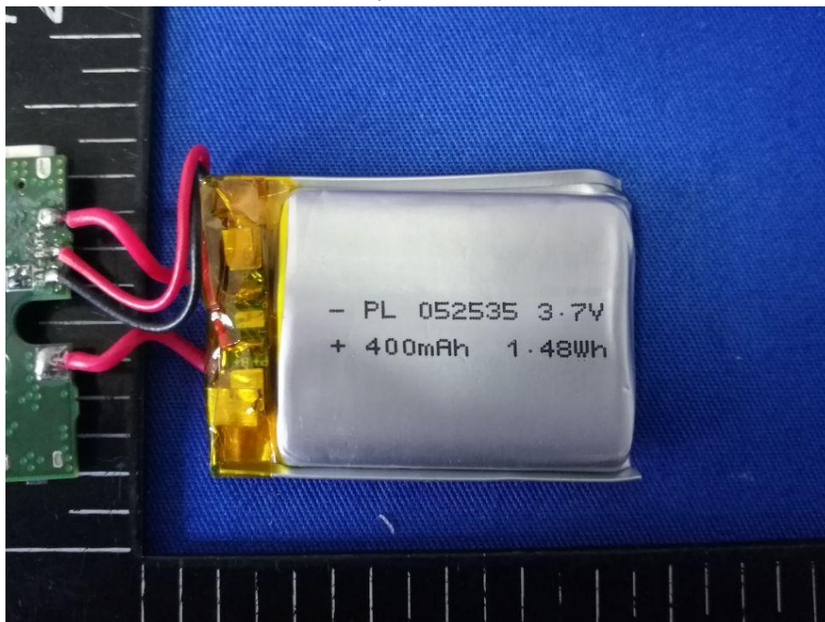
Battery - Front View
