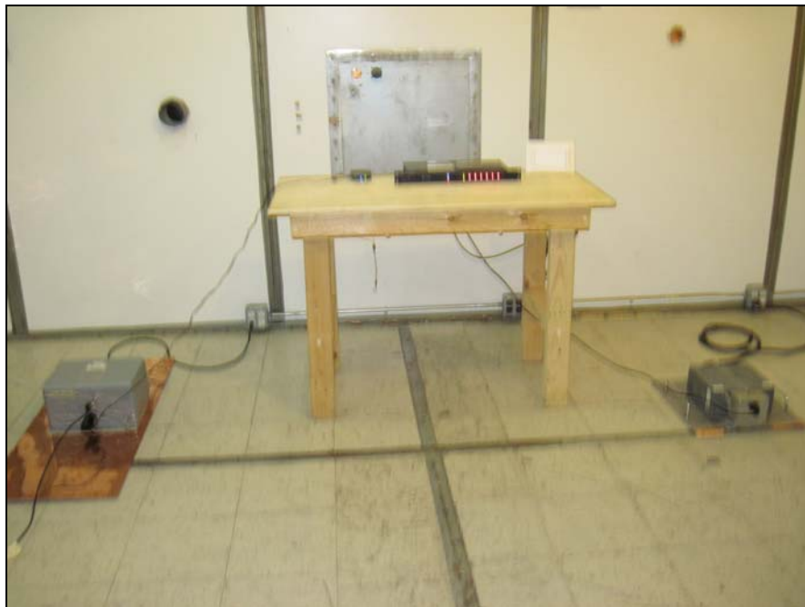
Photograph 3. Conducted Emissions, 15.207, Test Setup, Charging Mode
