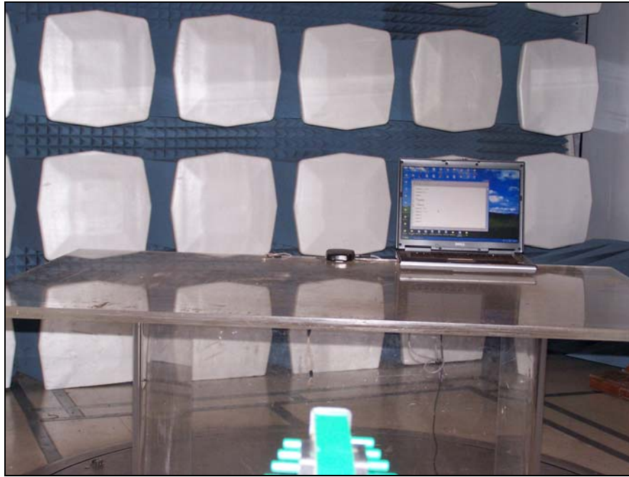
Photograph 5. Radiated Emissions, Test Setup, Class A Computer Peripheral
