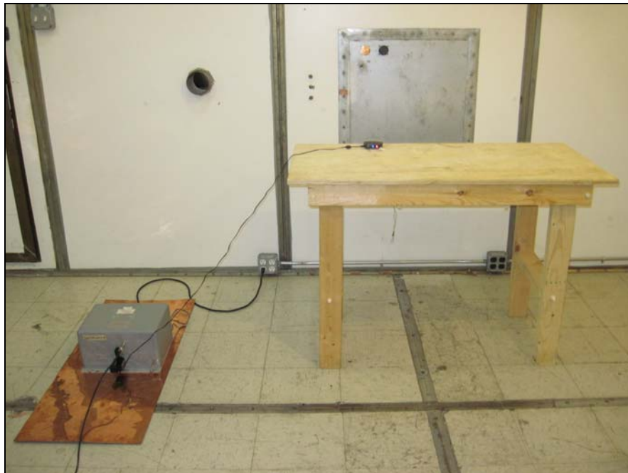
Photograph 2. Conducted Emissions, Test Setup, Charging Mode
