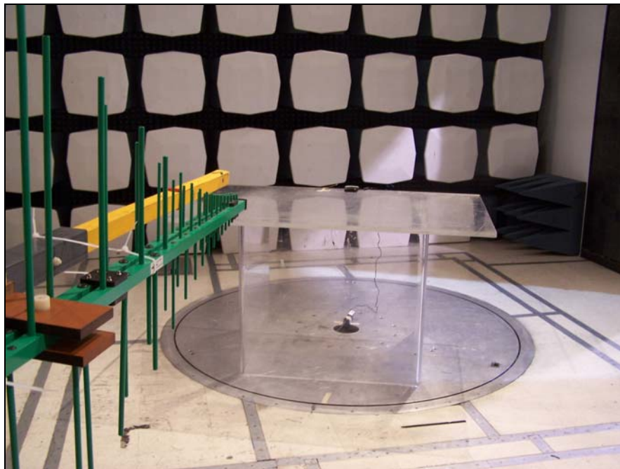
Photograph 4. Radiated Emissions, Test Setup, Charging Mode
