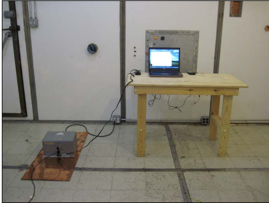
Photograph 1. Conducted Emissions, Test Setup, Class A Computer Peripheral
