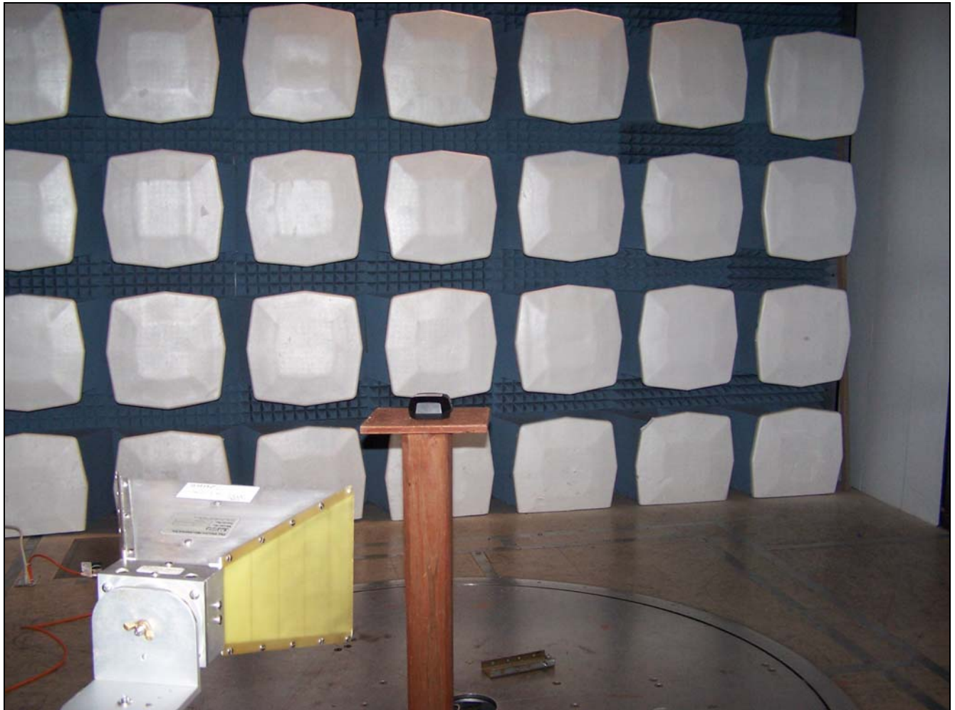
Figure 9. Radiated Emissions Test Setup
