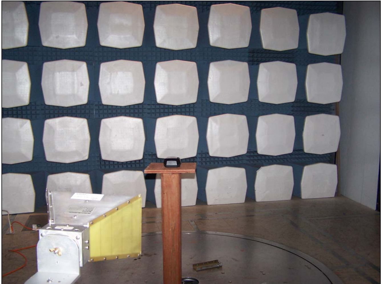
Photograph 4. Radiated Emission Test Setup - above 1 GHz
