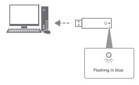
3. After pairing is complete, the indicator lamp of the headphones and transceiver light in blue
