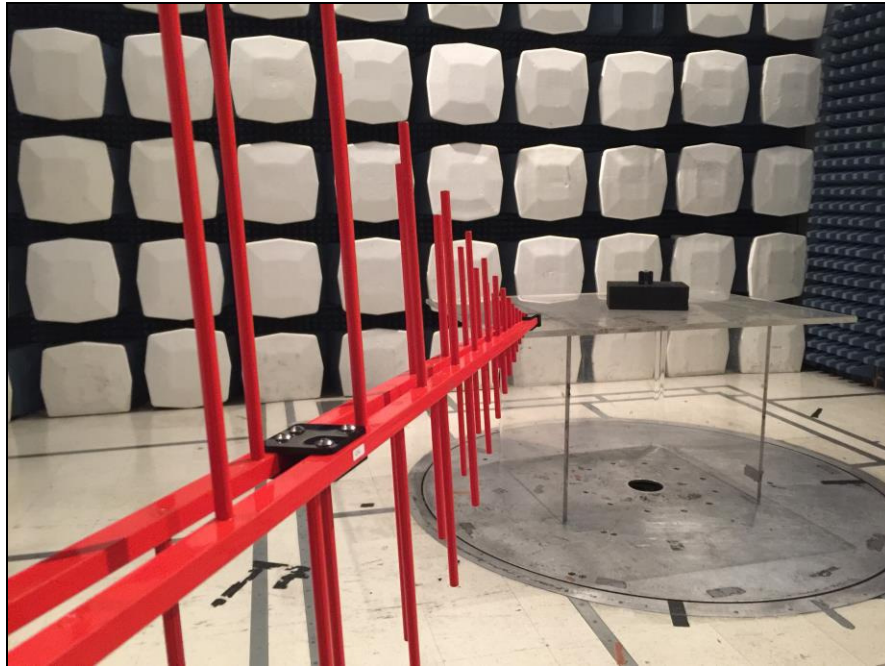
Photograph 1. Radiated Emissions, Test Setup, Below 1 GHz
