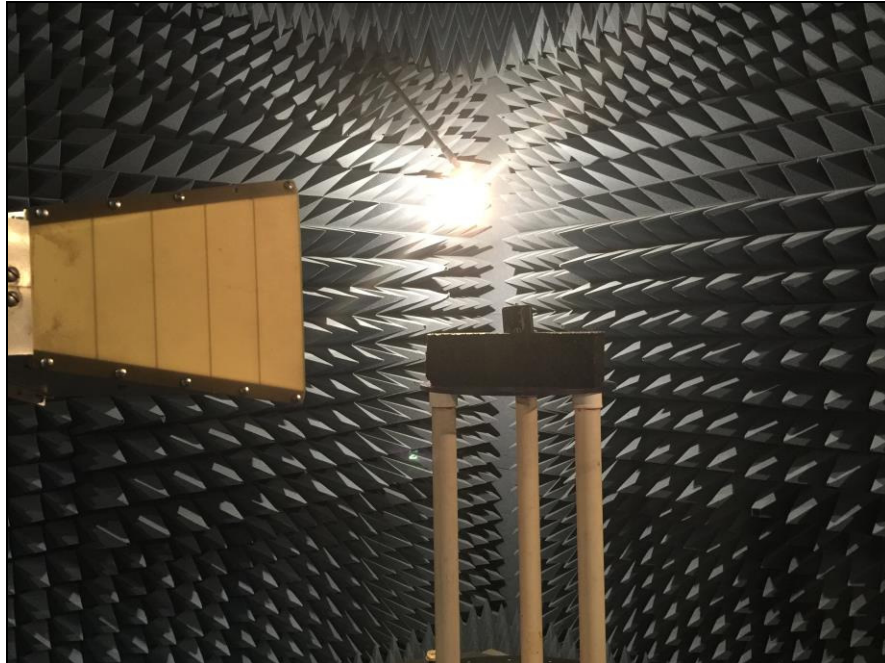
Photograph 2. Radiated Emissions, Test Setup, Above 1 GHz
