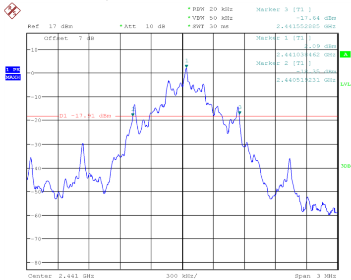
Fig.76 20dB Bandwidth: GFSK, Ch0
