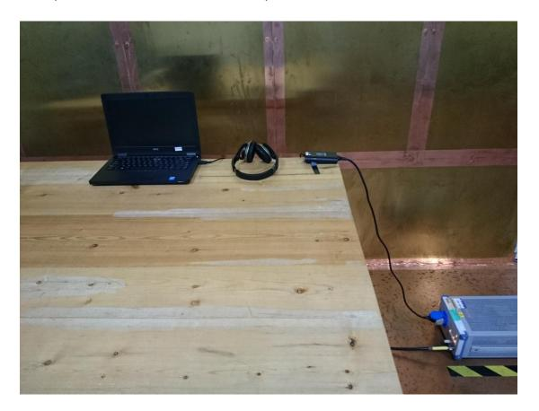
Description: Radiated Emission Test Setup (30-1000MHz)
