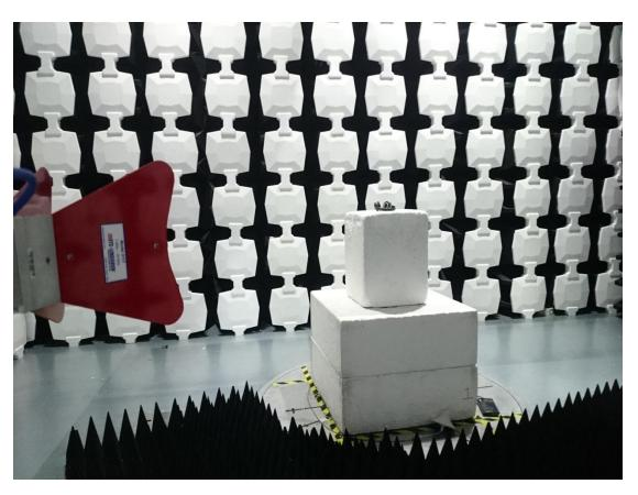
Description: Radiated Emission Test Setup (Above 18GHz)
