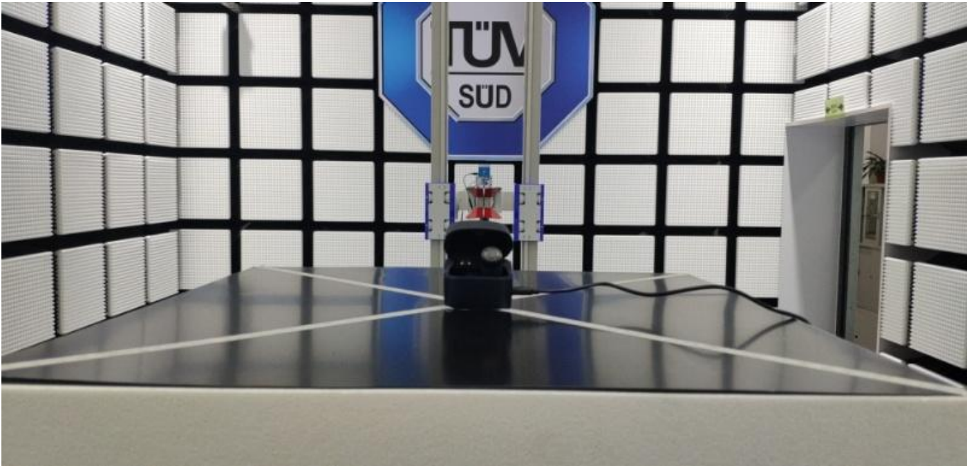
Radiated Emission Test 1GHz-18GHz
