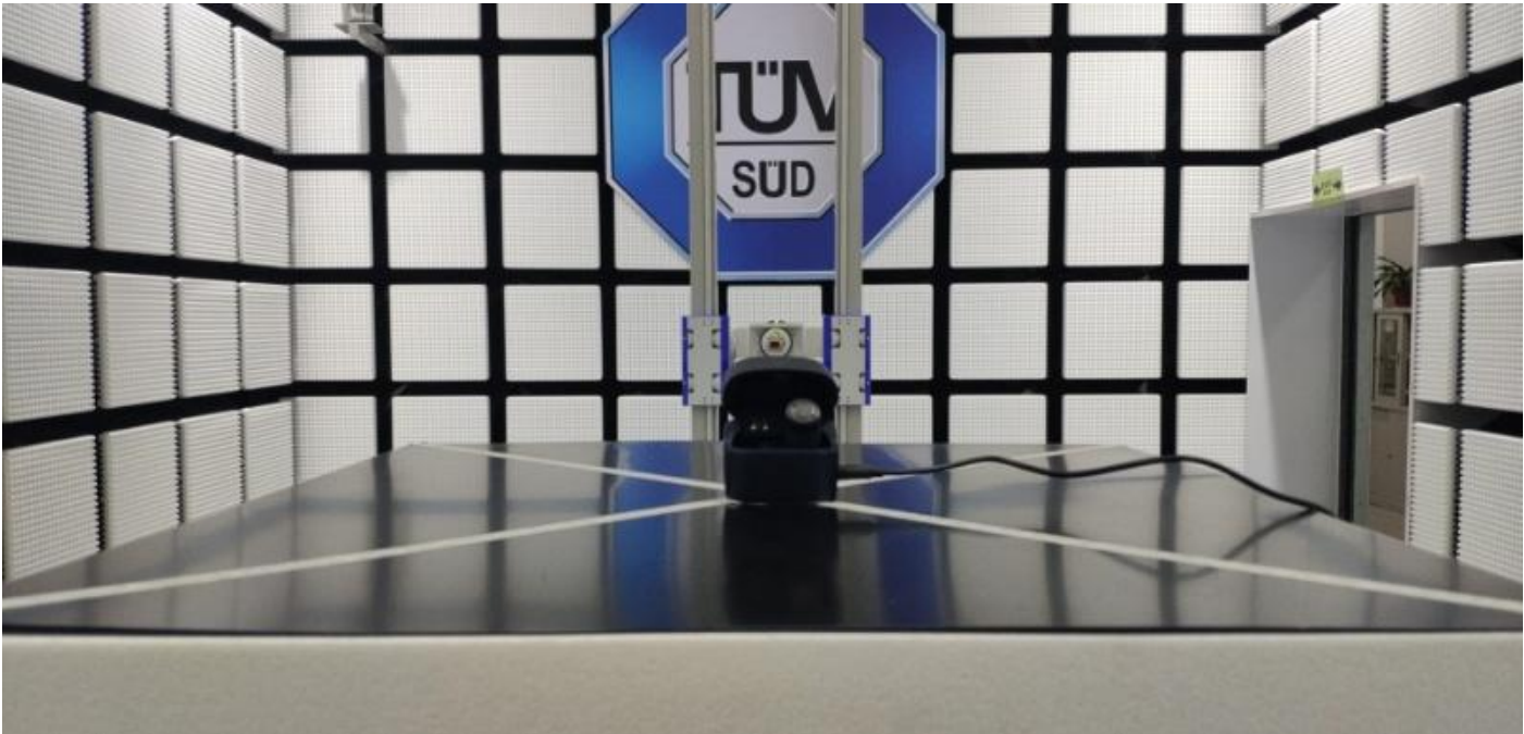
Radiated Emission Test 18GHz-40GHz
