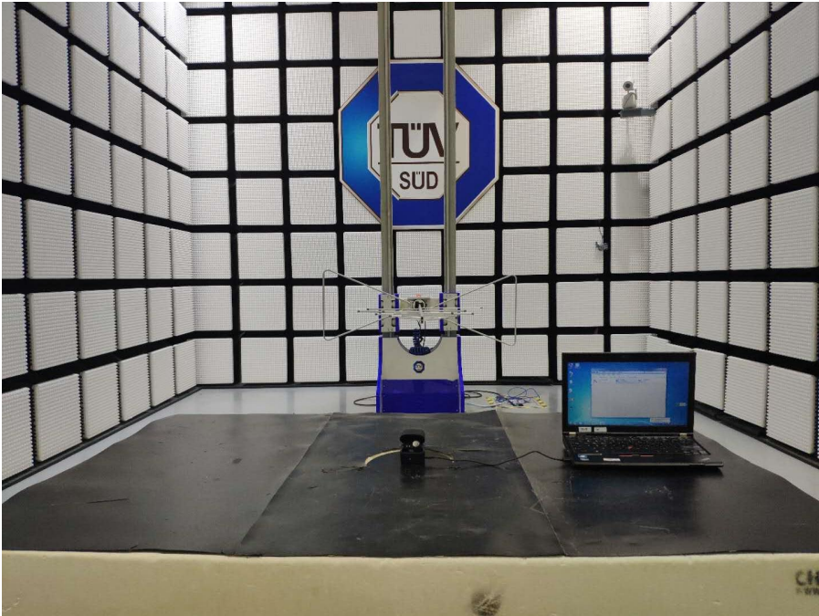
Radiated Emission Test 1GHz-18GHz
