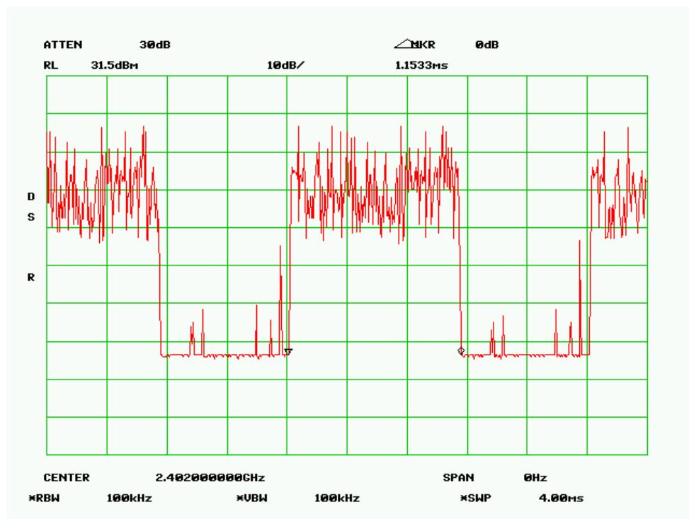
*Pulse width, 4 ms span*
