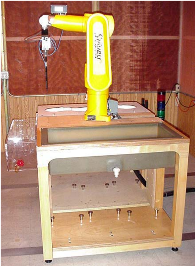
DASY4 SAR Measurement System with Planar Phantom
