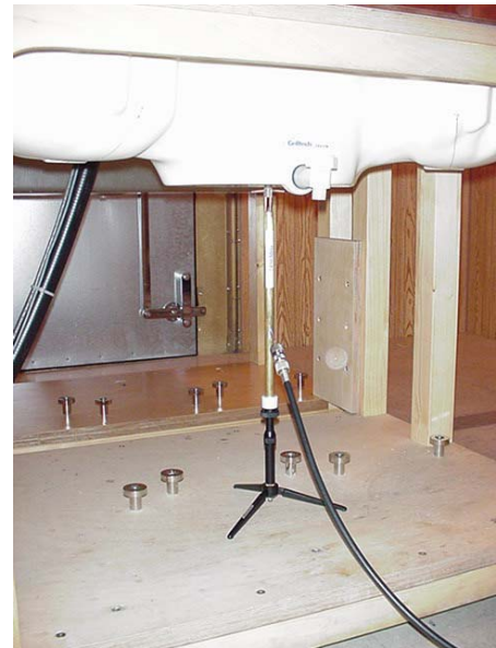
2450MHz Dipole Setup
