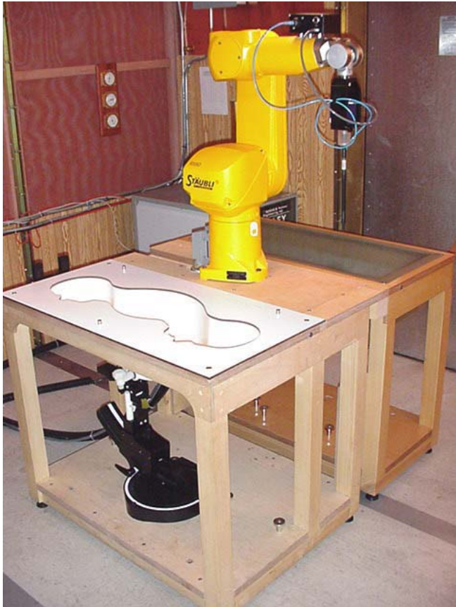
DASY4 SAR Measurement System with SAM Phantom
