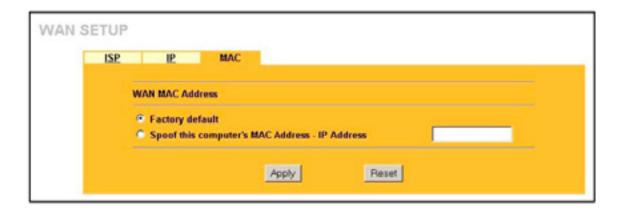
The MAC address screen allows users to configure the WAN port's MAC address by either using the factory default or cloning the MAC address from a computer on your LAN.
