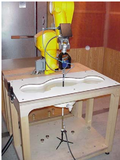
2450MHz System Performance Check Setup
