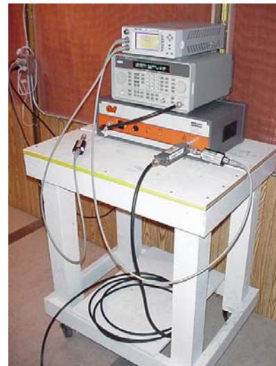
2450MHz System Performance Check Setup
