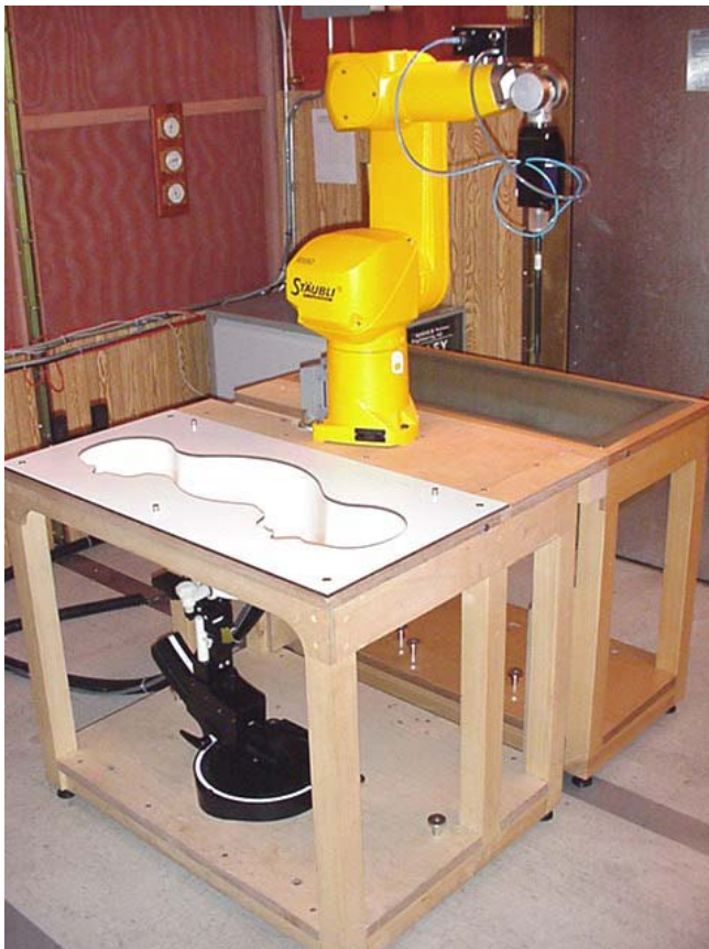
DASY4 SAR Measurement System with SAM Phantom
