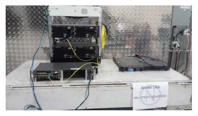
Rear of Powerline Conducted Emissions Setup
