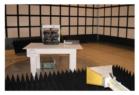
**Rear of Radiated Emissions Setup**
