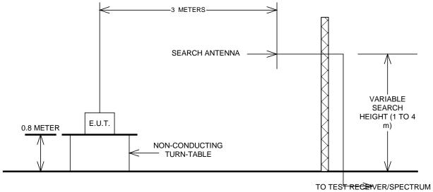
TO TES<sup>T</sup> REC₽IVER/SPECTRUM ANALYZER. A high-pass filter and LNA is necessary to measure to the limits of 15.209.
