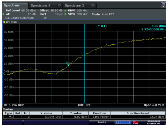
Figure 8.2-7: - Lower band edge emissions at 5725 MHz, 30 MHz Channel BW, Low channel
