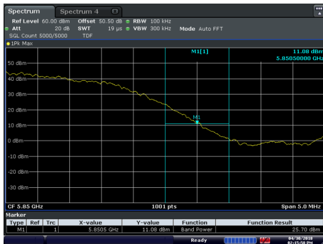
Figure 8.2-26: -- Upper band edge emissions at 5.850 GHz, 30 MHz Channel BW, High channel
