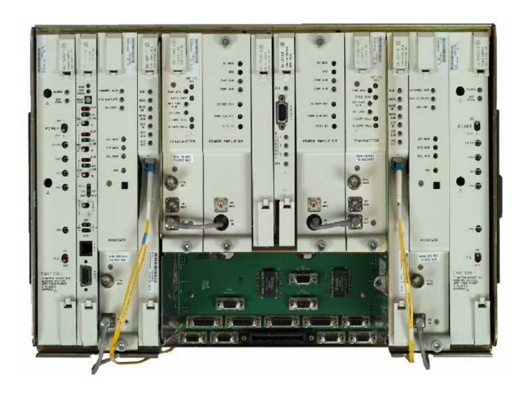
Figure 2–1 Typical MDR-8000/i/s/u Series Microwave Digital Radio
