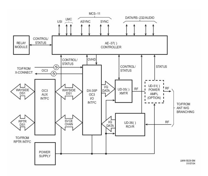
Figure 3-3 OC3 Non-Standby System Functional Block Diagram
