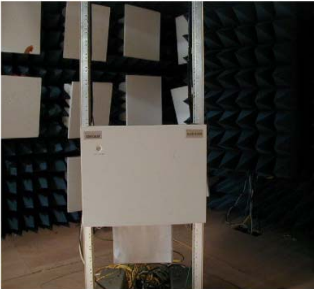
MDR8705u-XX radio mounted in a rack with over on.
