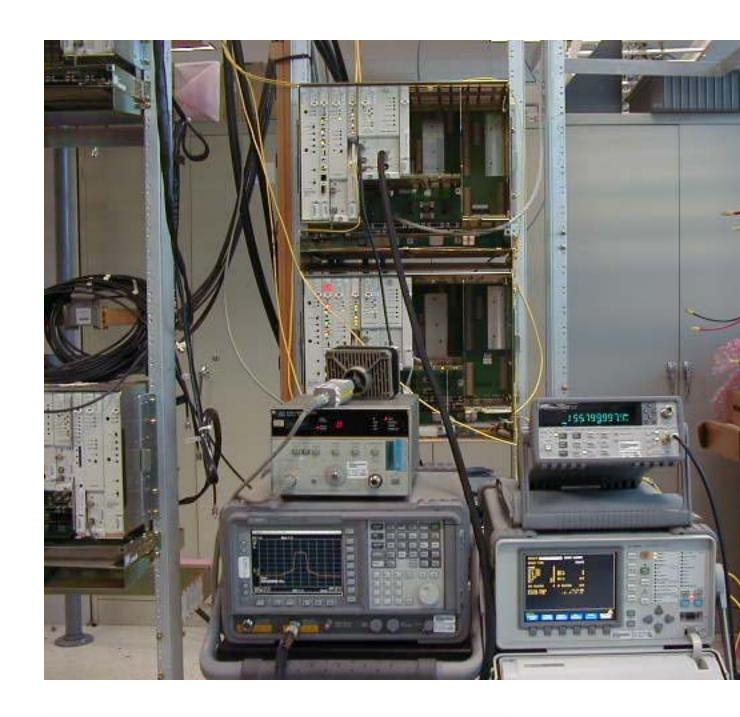
**Conducted Emissions Test Set-Up**
