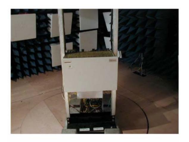
Radiated Emissions Test Set-Up
