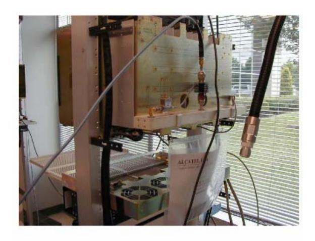
Conducted Emissions Test Set-Up (back view)
