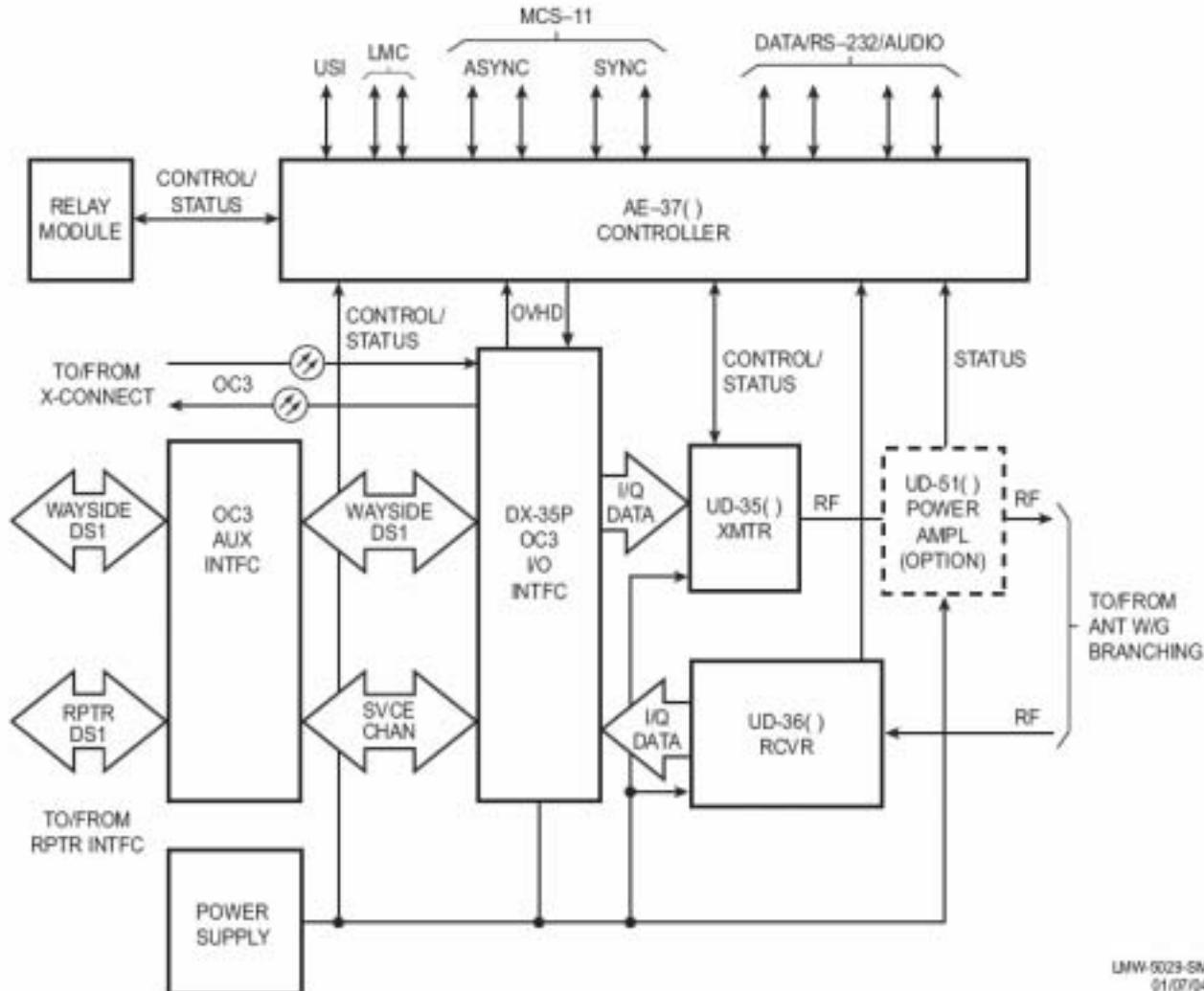
Figure 3-3 OC3 Non-Standby System Functional Block Diagram
