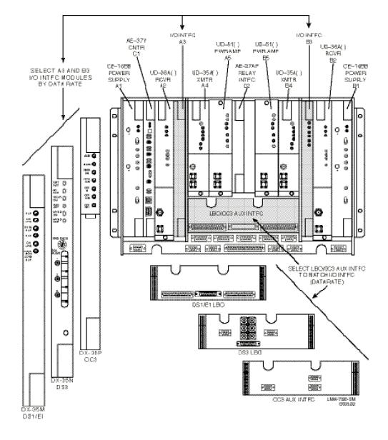
Figure 1 Typical MDR-8000 Hot-Standby Shelf Component
