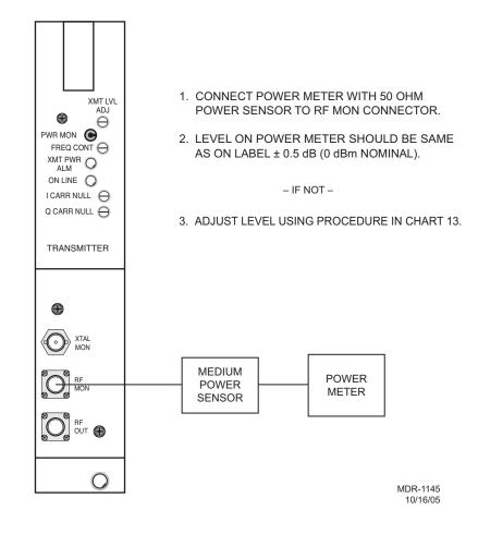
Figure 9-15 XMTR Output Level Check (No PA)
