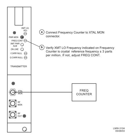
Figure 9-14 XMT Crystal Oscillator Frequency Check
