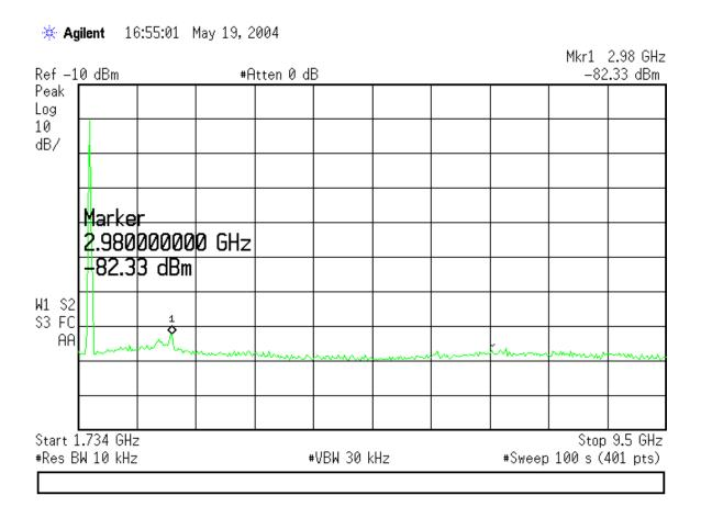
The power transmitted here is 1 Watt. This measurement was taken at the antenna port of the FR filter. The RF filter has at least 90 dB of rejection at the second harmonic. We had to notch the fundamental frequency to make this measurement but we did not affect the harmonics. I think this is all of the tests you requested. If I left out anything just let me know.
