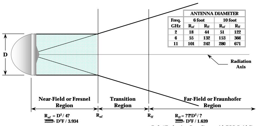
**R**<sub>nf</sub> = Distance from the antenna to Near-Field boundary (ft).
