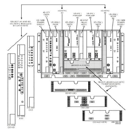
Figure 1. Typical MDR-8000 Hot-Standby Shelf Component
