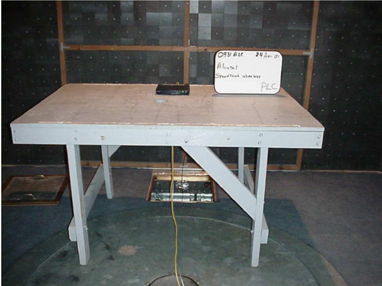
Figure 4 - Conducted Emissions Test Setup (Front)
