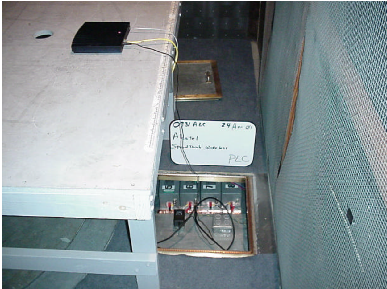
Figure 5 - Conducted Emissions Test Setup (Back)
