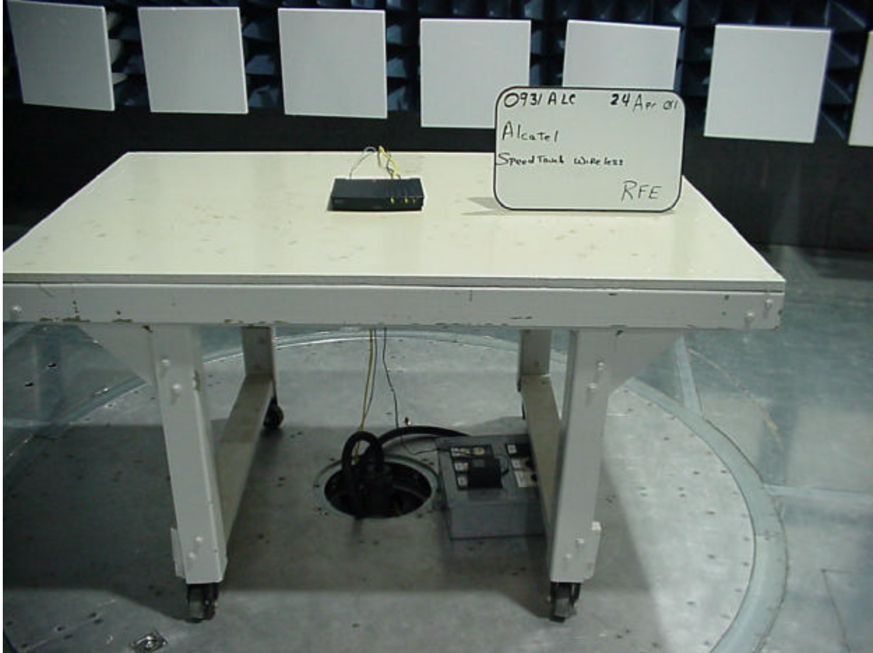
Figure 2 - Preliminary Radiated Emissions Test Setup (Chamber - Front)
