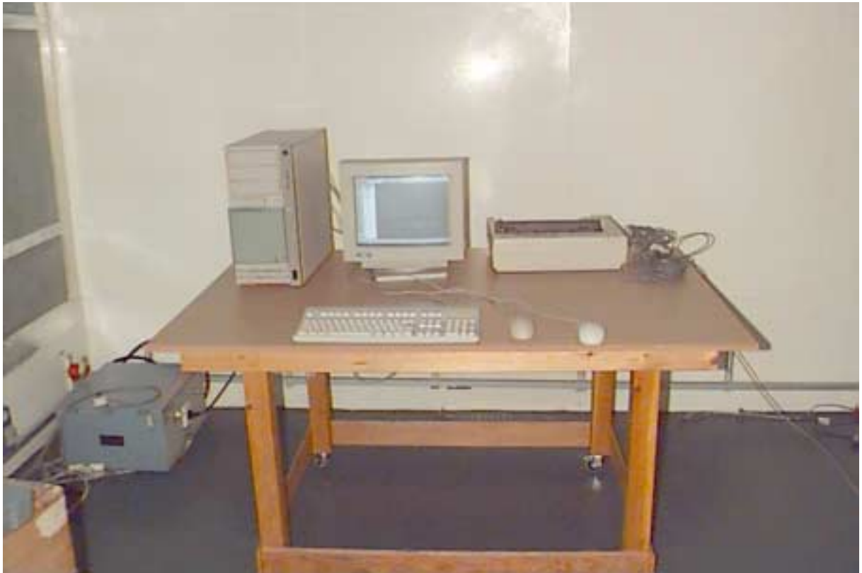
Photograph No.6 Conducted emissions measurement setup at 120 VAC port of PC
