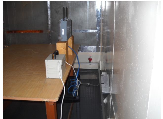
Photograph 8.1.1 Setup for conducted emission measurements
