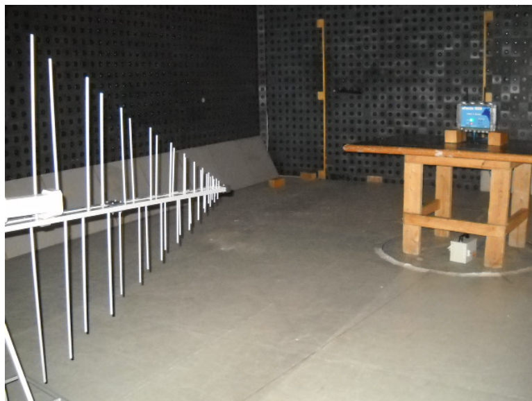
Photograph 8.2.1 Setup for radiated emission measurements
