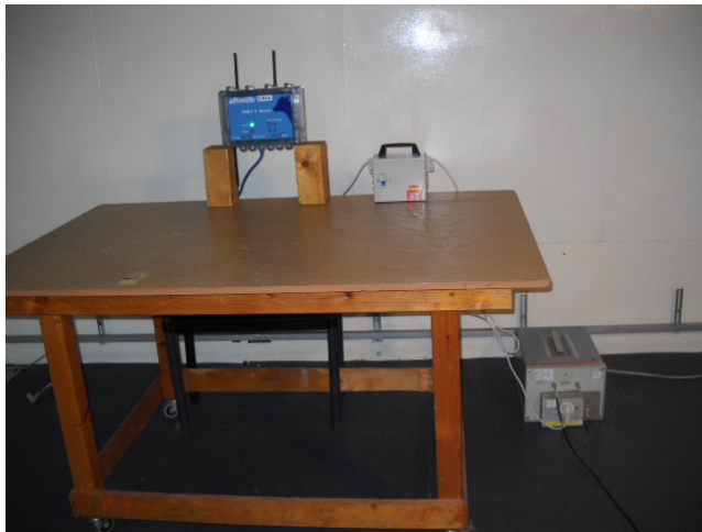
Photograph 8.1.1 Setup for conducted emission measurements
