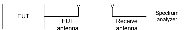
Figure 7.4.1 Occupied bandwidth test setup
