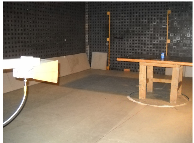
Photograph 8.1.1 Setup for radiated emission measurements
