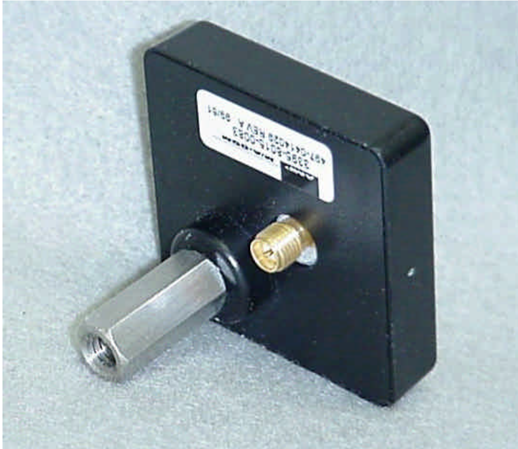
Photo 17. Bottom View of Transmit Antenna (Passive Patch)
