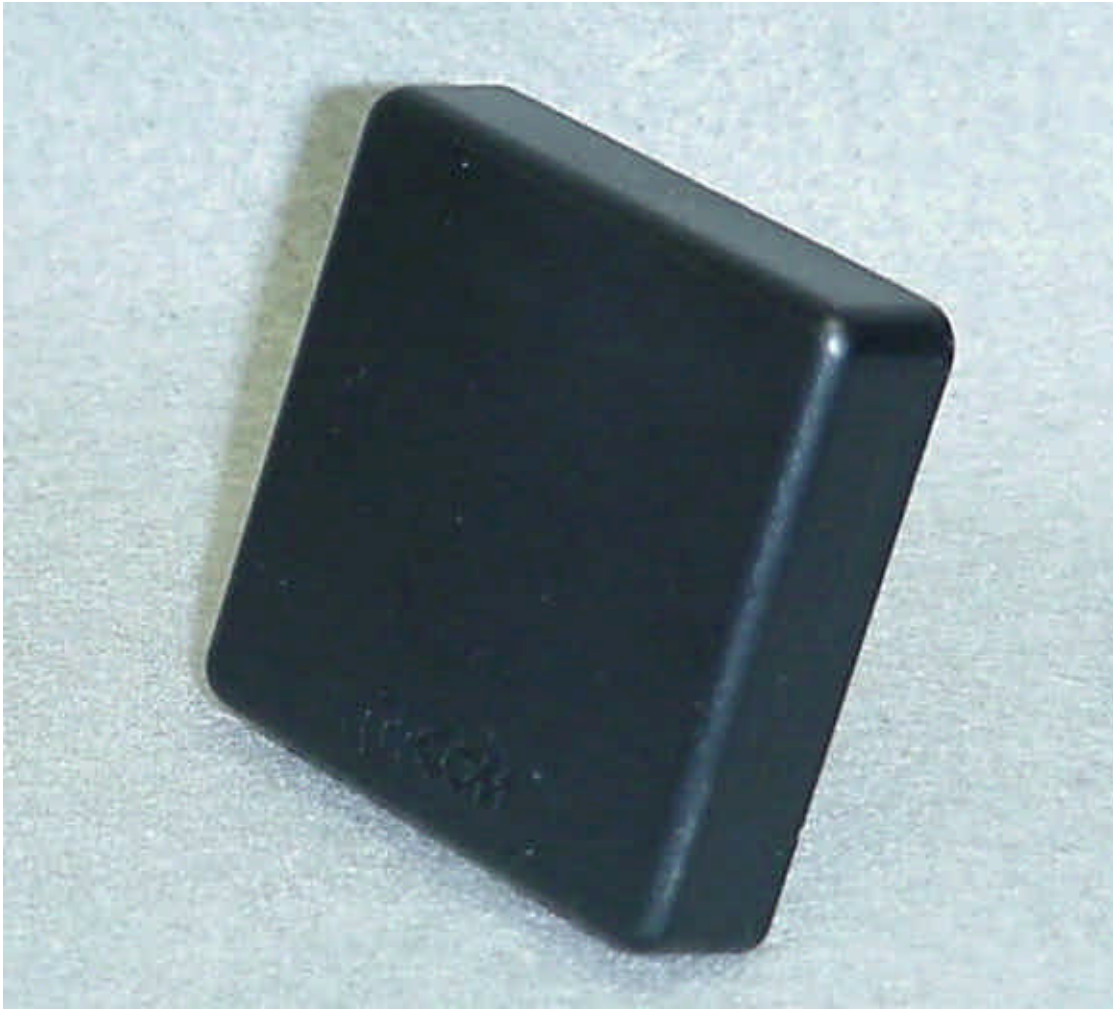
Photo 16. Top View of Transmit Antenna (Passive Patch)
