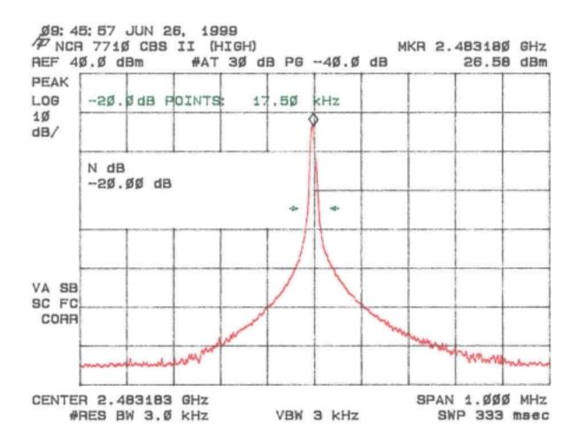
Figure 7c. 20 dB Bandwidth per FCC Section 15.247(a)(1)(ii) (High)
