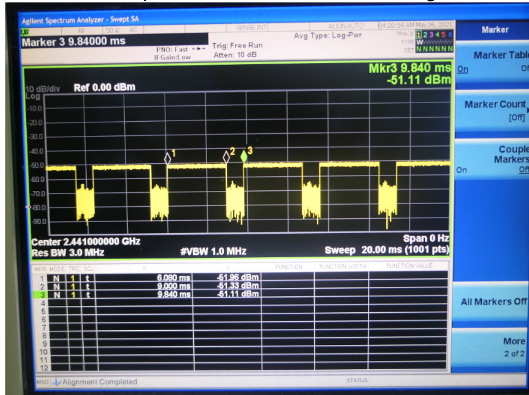
Time-domain plot for Bluetooth transmission signal
