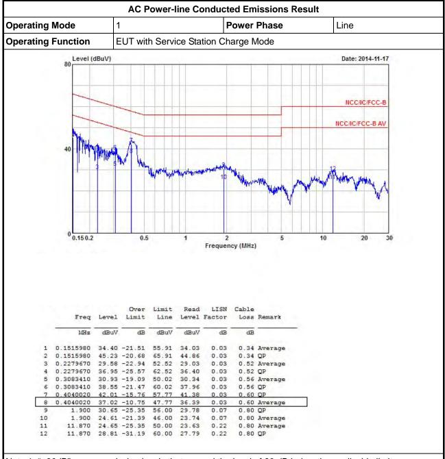
Note 1: ">20dB" means emission levels that exceed the level of 20 dB below the applicable limit. Note 2: "N/F" means Nothing Found emissions (No emissions were detected.)
