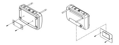
To combine two receivers in a 19" standard rack by using 2 short L type plastics racks (L2) and 2 metal connecting plates (C1). (Each system includes a L2 and a C1.)
