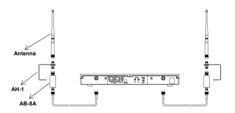
Antenna holder makes it easy to fix wherever for connection antenna and booster. AH-1 can be assembled on the mic stand or on the wall.
