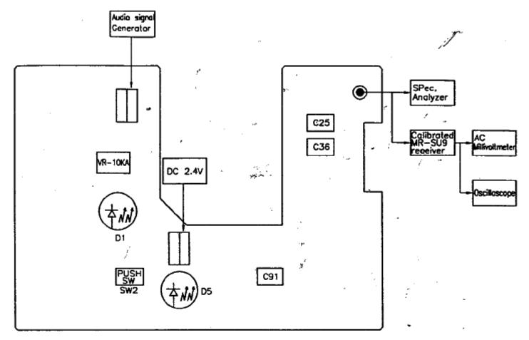
Definition of "calibrated MR-SU9 receiver" calibration:RF-INPUT:48KHZ deviation at 1KHZ audio-frequency+Tone key calibrate output voltage with AF-out to 0dBV±0.05dB
