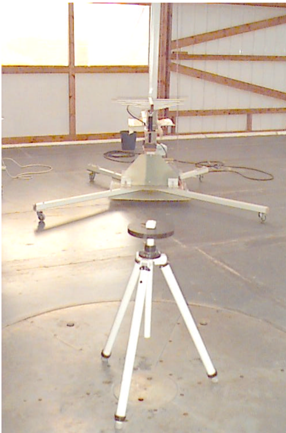
Photograph 2 Radiated emissions measurement test setup
